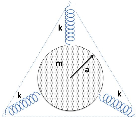
A uniform disk of mass  $m$  and radius  $a$  rests on a horizontal frictionless surface. It is symmetrically attached to three identical, ideal, massless springs of spring constant  $k$  whose other ends are attached to the three vertices of an equilateral triangle.
