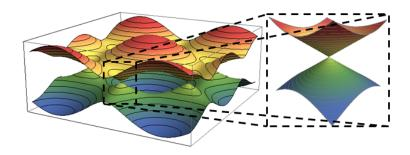
The figure shows the allowed energies in a graphene lattice. Our energy relation comes from approximating the surface to be a cone near lattice points, in k-space. This is called the Dirac cone in literature. It has slope  $v_F$ , dimensions [p/m], and is called the Fermi velocity.
