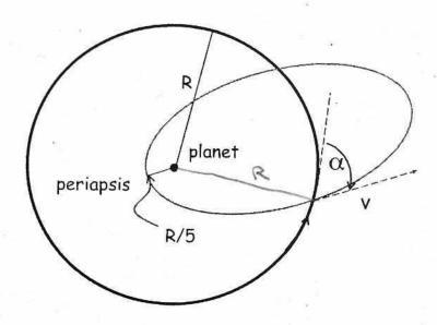
At a specific point in the satellite's circular orbit, the velocity of the satellite is abruptly rotated without changing the magnitude of its velocity. (The nature of this external impulse is not specified.) As shown in the figure, this causes the satellite to enter an elliptical orbit with its distance of closest approach = R/5. (This point in the elliptical orbit is called the periapsis in general.) The elliptical orbit is in the same plane as the circular orbit.
